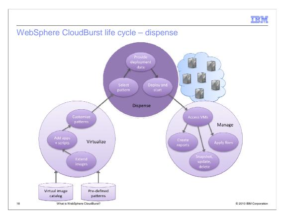
This sub-section focuses on the "Dispense" phase of the life cycle. In this phase, once the pattern is selected and customized, the deployment parameters are entered to create the virtual systems. These virtual systems are then deployed onto hypervisors in the cloud.
