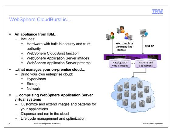
WebSphere Cloudburst is a hardware appliance that provisions hardened WebSphere Application Server topologies into a cloud of virtualized hardware. The appliance contains WebSphere Application Server virtual images and patterns. Your own hardware is used to create the cloud into which application server virtual images are dispensed and managed by the appliance.
