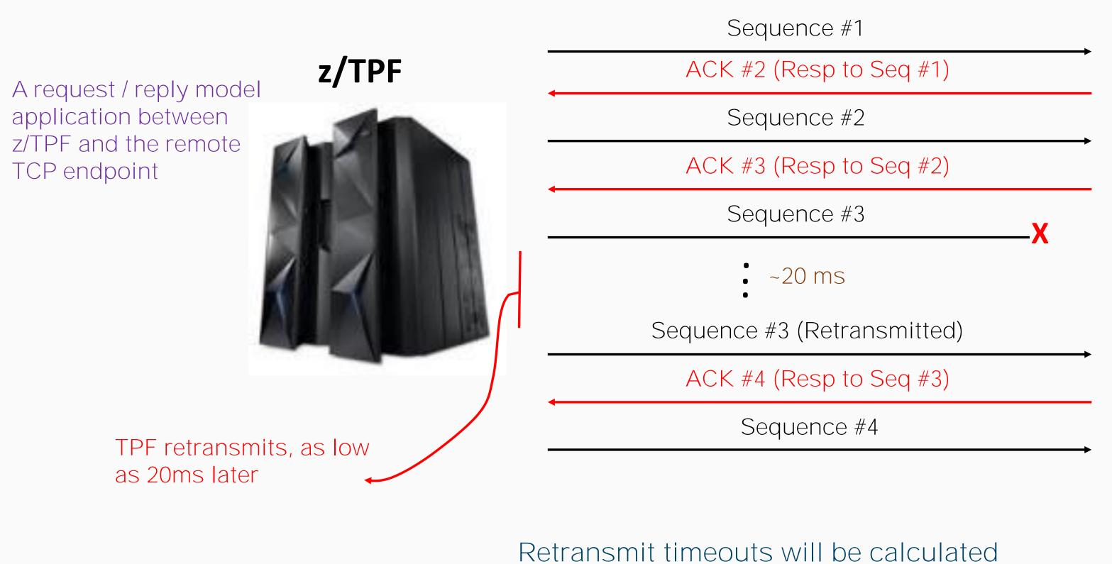
Retransmit timeouts will be calculated from **socket's round** trip time (RTT) and variance of it (RTTVAR).
