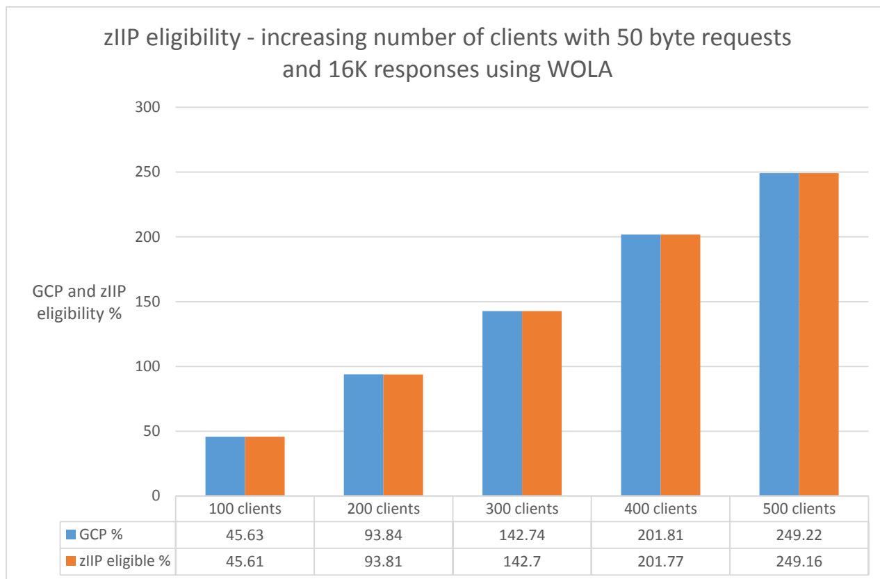
Figure 25 GCP CPU % and zIIP eligibility for increasing numbers of clients with 16K responses
