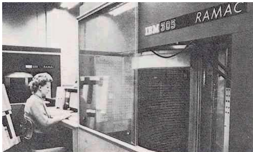
The world's first disk storage system, the IBM 350 Disk Storage Unit (in the IBM 305 RAMAC computer), with 5 megabytes capacity, was introduced in 1956.
