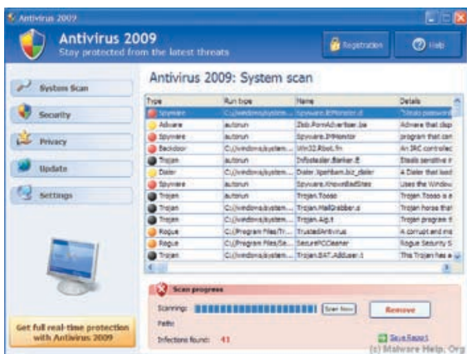
Figure 50: An example of fraudulent malware touting antivirus protection. Even if the user does not click the “Continue” button, a rogue security software will still be downloaded and installed.
