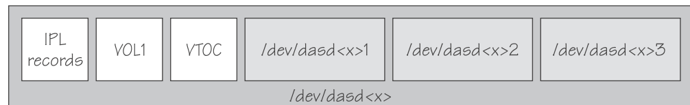
Figure 31. Compatible disk layout
