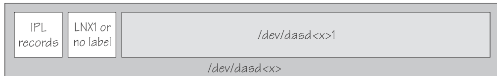
Figure 32. Linux disk layout
