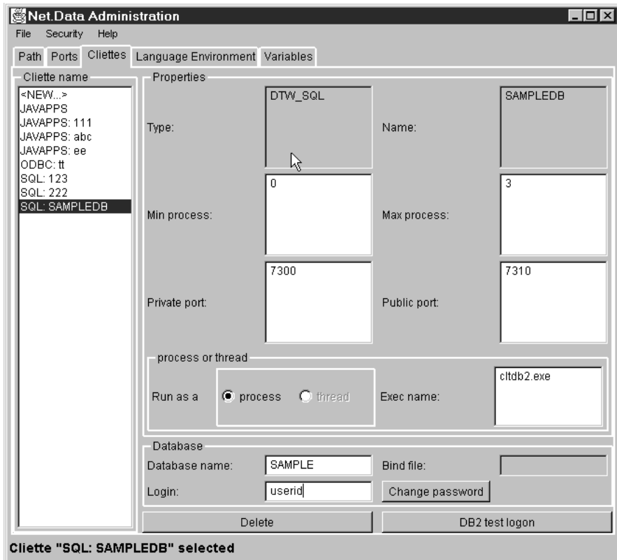
Figure 9. The Cliette Page of the Net.Data Administration Tool. Use this page to add, modify, and delete cliettes.
