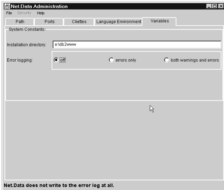
Figure 14. The Variables Page the Net.Data Administration Tool. Use this page to specify initialization variables.
