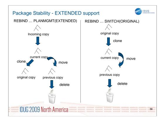
•This diagram shows the EXTENDED support. The previous copy is thrown to the trash can. The current copy becomes the precious copy. Only the first time you execute this, when we don't have the original copy stored, do we take the current copy and store it as the original copy. And the newly generated copy becomes the current.
