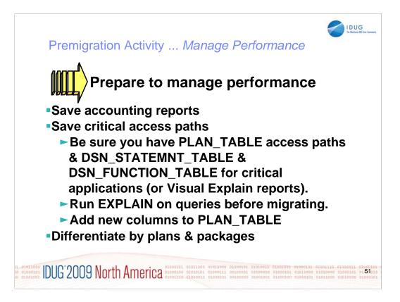
Save critical access paths & accounting data! Changes can cause unwanted access path changes. Identify important queries, plans & packages. Be sure plan tables contain access paths & costs. ALTER current plan tables to add new columns. EXPLAIN REBIND may change access paths, so extract plans & run EXPLAIN under a dummy collection, a different application or program name.
