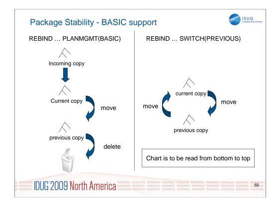
•The diagram shows the scenario of BASIC support. It is to be read bottom up. At the left hand side, when you rebind using PLANMGMT(BASIC), we discard the previous copy, take the current copy and store it as the previous copy, and take the newly generated copy as the current copy.
