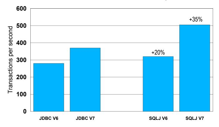
Normalized throughput for zSeries G7 with 3 engines with 100% cache hit for JDBC. SQLJ advantage increased from 20% to 35% when Java overhead was reduced.
