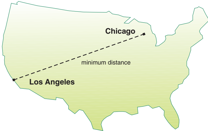
Figure 25. Minimum distance between two cities. The function ST_Distance can take the coordinates for the locations of Los Angeles and Chicago as input, and return a value denoting the minimum distance between these locations.
