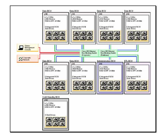
The preceding diagram gives an impression of a small BCU configuration which has all options enabled. It is important to see that the cluster management console is actually nothing else than any workstation connection to the administrator BCU or simpler to the coordinator node of the cluster. Unlike typical high performance computing clusters such as Linux Beowulf clusters, DB2 UDB for Linux does not need an additional management or head node.
