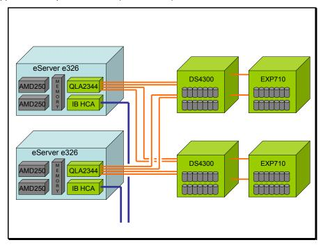
Each server has a theoretical fibre channel throughput of 600 MB/sec. Various benchmarks have demonstrated that the server actually can operate at this throughput for a sustained period of time. Each of the DS4300 storage controllers can be active with one server at a time to deliver the full 300 MB/sec throughput per each storage system. The redundant connections between the DS4300 and the EXP710 offer additional reliability for the system.
