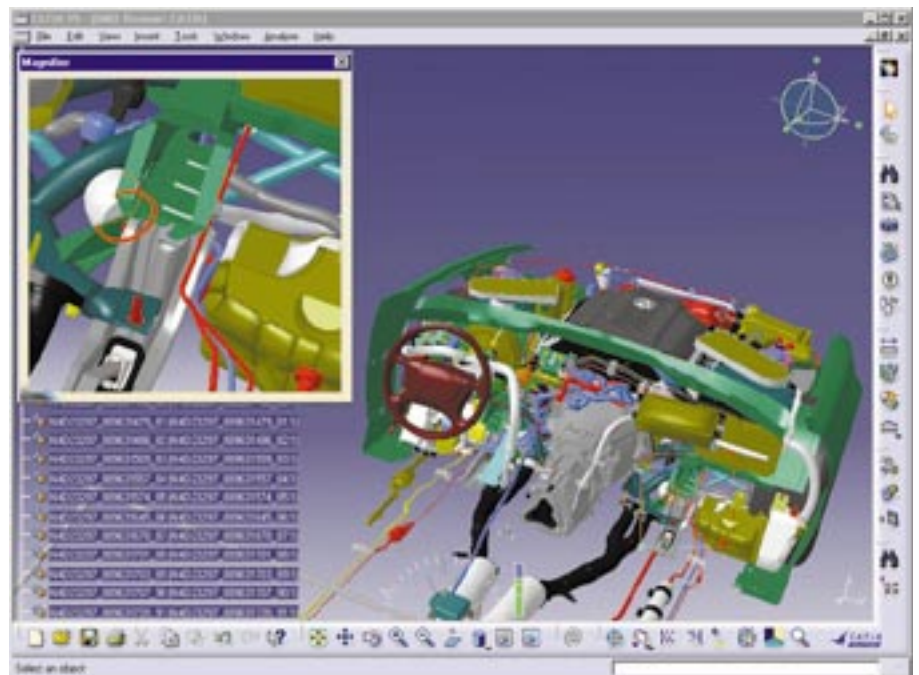
Integrated navigation and review tools enable users of CATIA to “fly through” 3D digital mock-ups early in the design cycle.
