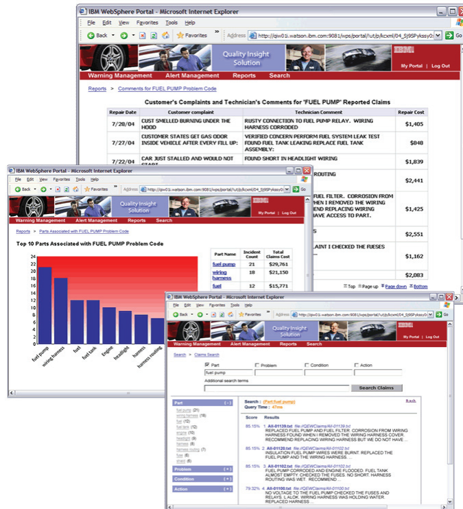
Figure 17: Issues Analytics and Quality Early Warning Applications can deliver richer reports that identify other parts involved in a problem and provide an understanding of the actual conditions that cause failures.
