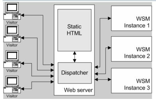
But the dispatcher does even more: You can split up the dynamic parts to different servers, so you gain additional processing power, the server is fail-safe, or you can manage different Web sites on the same static Web server. All of these techniques are summarized as "load balancing". It means that servers can share their work seamlessly. The dispatcher allows for a number of very useful load balancing scenarios.
