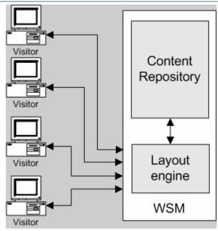
If you use a Content Management Server, such as FileNet WSM, an advanced layout engine processes the request from a visitor. The engine reads content from a repository and uses styles, formats and access rights to transform the content into a document that is tailored to the visitor's needs and rights.
