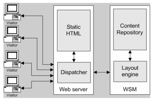
The dispatcher works as part of a static HTML server, such as Apache. The aim of the dispatcher is to store (or "cache") the Site content as much as possible in the form of a static Web site, and access the layout engine as little as possible. This approach brings you the best of two worlds:
