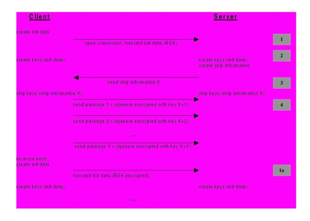
Figure 4-1. Encrypted Client-Server communication.
