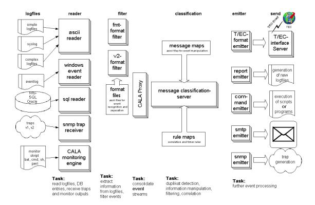
This open architecture enables CALA to be implemented at almost any desired level of complexity or heterogeneity.
