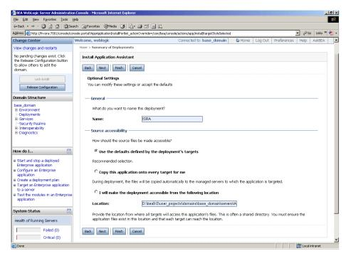
This screen displays the optional settings of the deployed file.
