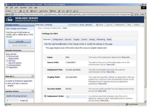
An overview of the deployments made is reflected. The **ISRA.jar** file is successfully deployed.
