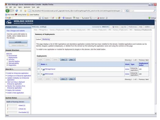
The system returns to the Deployment page, showing ISRA is undeployed.
