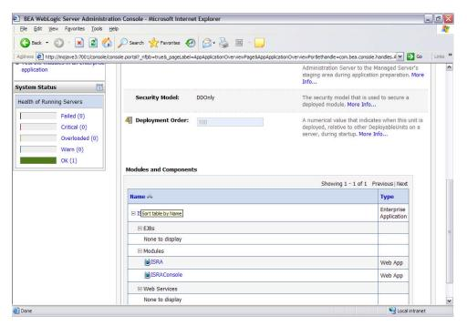
An overview of the deployments made is reflected. The **ISRAConsole.ear** file is successfully deployed.
