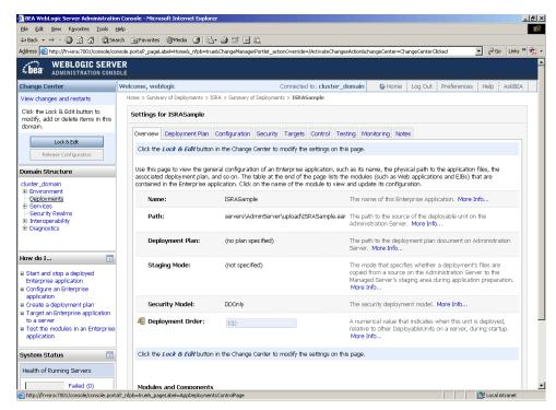
An overview of the deployments made is reflected. The **ISRAConsole.ear** file is successfully deployed.
