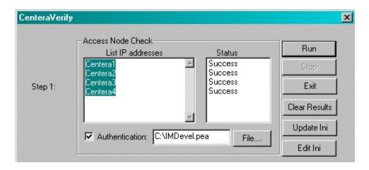
The first step in the Centera Verify program verifies that it can access each Centera device successfully.
