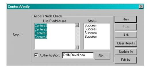
The first step in the CenteraVerify program verifies that it can access each Centera device successfully.
