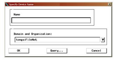
2 Enter the device name in the Name field or click Query to search for the device name. See "Using the Query Feature to Select a Device Name" on page 101.
