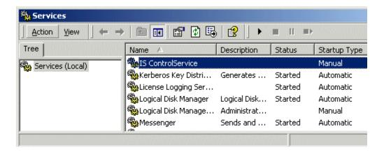
3 In the list of Services, verify that IS ControlService is Started with Startup Type set to *Automatic*. (If the service is not started the TM daemon is not running.)
