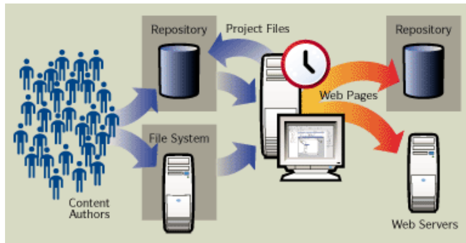
Figure 4-1 You can add source files from FileNet Content Manager or FileNet Content Services to a project and publish back to the repository or directly to a web server. You can also save project files in the FileNet repository.
