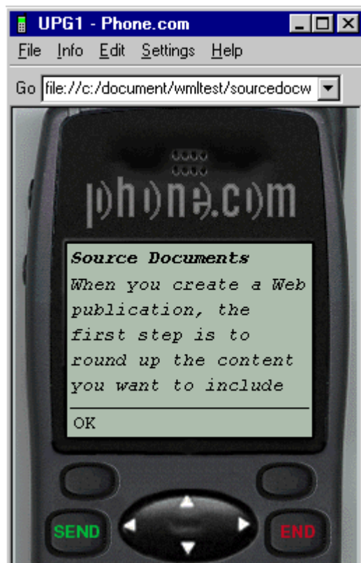
Figure 1-9 By typing "File://" plus the path for your output WML file on your hard drive in the Go field, you can view your WML output in your micro browser.
