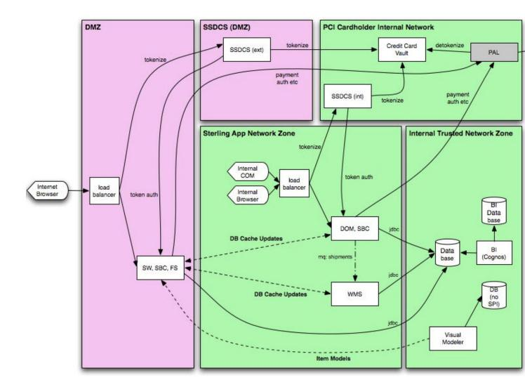
In this deployment strategy, you must open up firewall ports to allow inter-application communication between the Sterling Call Center and the Sterling Distributed Order Management applications.
