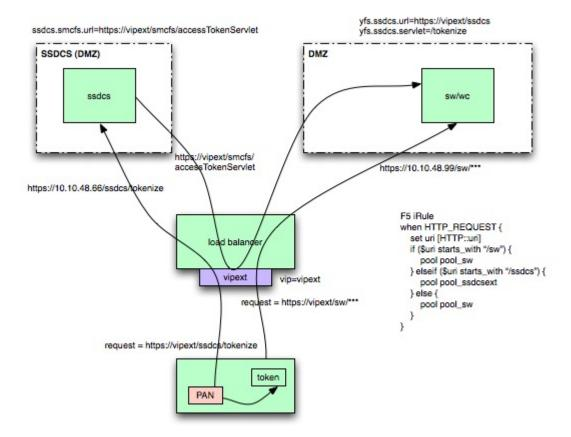
In the diagram, requests from the browser are sent to a load balancer to the virtual IP (VIP) https://www.acme.com. The load balancer is configured to route the traffic to either the SSDCS or Sterling Selling and Fulfillment Suite™ applications based on the URI shown to the right of the host and port. For example, if the load balancer is an F5 Big-IP, you could set up the following iRule to route requests to the appropriate load balancing pool (of servers) based on the URI.
