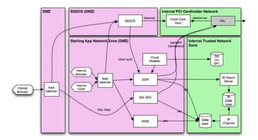
The Sterling Distributed Order Management, Sterling Web, and Sterling Field Sales applications are placed into a security zone: the Sterling Application Network Zone (SANZ). Optionally, you can then add the Sterling Warehouse Management<sup>TM</sup> System, which has the same inter-application communication requirements as the other applications, into the SANZ.
