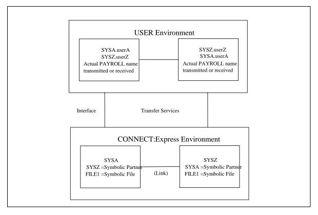
To transfer PAYROLL files between userA on SYSA and userZ on SYSZ, you must define SYSA and SYSZ as Partners and create the common FILE1 definition in Connect:Express directories. Connect:Express uses only the symbolic names when processing the transfer, and provides the interface through which user information is moved in both directions.
