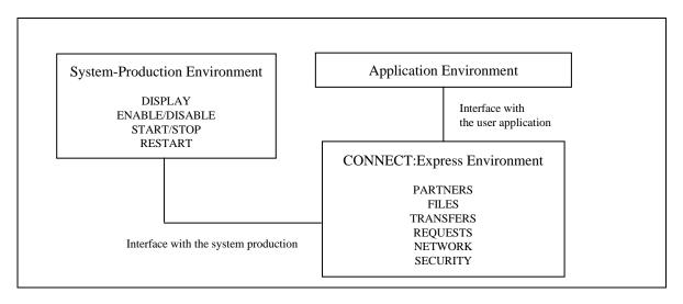
Transfer protocols enable applications to exchange specific information. Connect:Express provides transfer services through interfaces that establish communication between applications, as shown in the following illustration.
