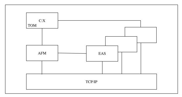
The following diagram shows the relationship between the Auxiliary FTP Manager (AFM), the EAS, and the Connect:Express user interface.
