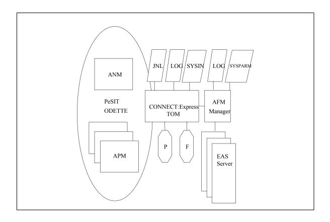
The Auxiliary FTP Manager modules communicate with each other and with Connect:Express using cross memory services.
