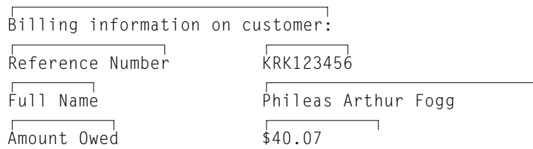
Figure 53. Part of a formatted screen, showing fields. Each block of text on the screen is a separate field. The fields on the left were filled in by program; those on the right were completed by an operator.
