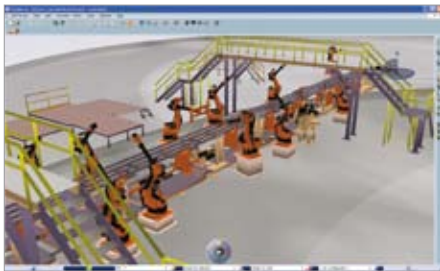
DELMIA—3DLive displays the manufacturing resources and work stations stored in the Manufacturing Hub in 3D.
