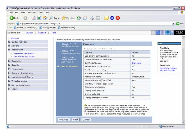
Check the settings on this page and select <u>Finish</u> to start the installation of your application. When the installation of the application has been completed it must be <u>saved</u> in the master configuration.
