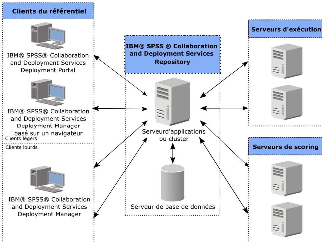
Figure 1. IBM SPSS Collaboration and Deployment Services Architecture
