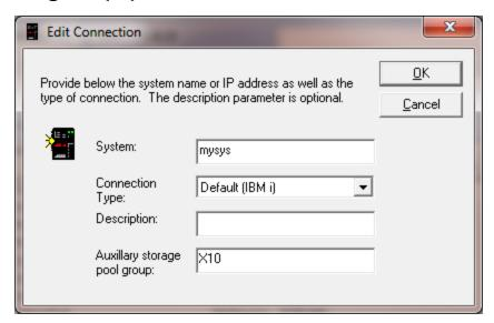
ASP group value used must be the IASP database name shown in System i Navigator and the ASP group name shown in WRKDEVD \*ASP
