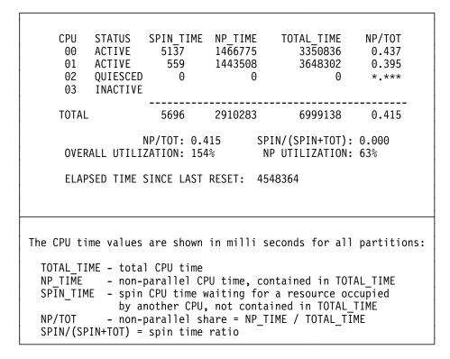
Figure 46. QUERY TD Output Example
