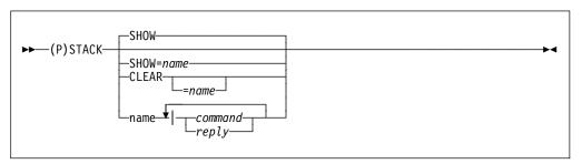
Figure 34. STACK command syntax
