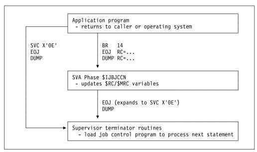
Figure 56. Normal Termination of an Application Program
