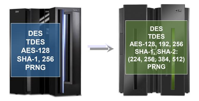
If you plan to enable CPACF, consider that it can only be enabled or disabled on a per central processor complex (CPC) basis and will affect all logical partitions (LPAR). The CPACF feature code is 3863. For information about how to enable a feature code see System z10 Support Element Operations Guide, SC28-6979.
