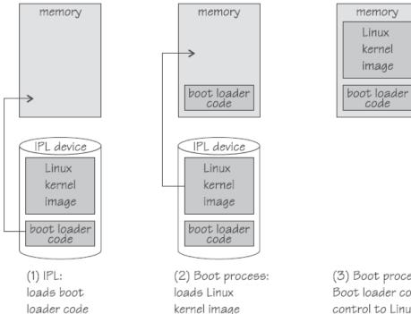
(3) Boot process: Boot loader code passes control to Linux
