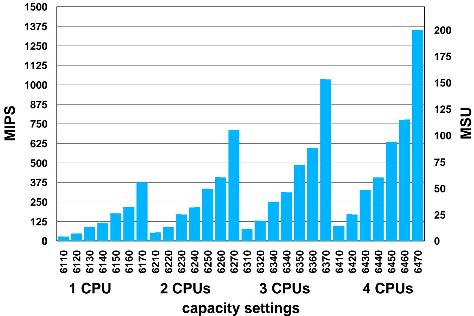
z890 consists of one Model (A04) and 28 capacity settings
