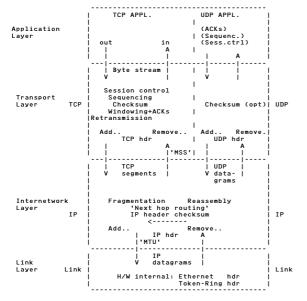
Outbound fragmentation may occur if MTU-40byte < MSS of other system Inbound reassembly may occur if MTU-40byte < MSS of VSE host
