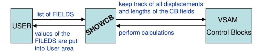
The first part of the enhancement extends SHOWCB to enable monitoring of VSAM LSR datasets using an officially supported API.
