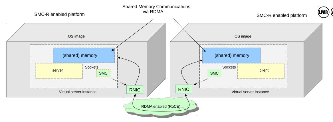
RDMA technology provides the capability to allow hosts to logically share memory. The SMC-R protocol defines a means to exploit the shared memory for communications - transparent to the applications!
