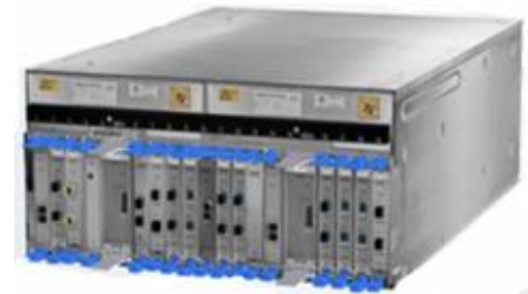
PCIe I/O drawer 32 I/O slots
