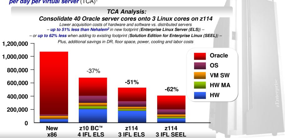
Based on US Enterprise Linux Server pricing. Pricing may vary by country. Model configuration included 10 IFL cores running a mixed workload averaging 31 virtual machines per core with varying degrees of activity. Includes zEnterprise hardware and z/VM virtualization software. Does not include Linux OS or middleware software.
