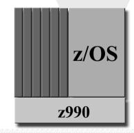
Up to 32 Central Processors Up to 256 Real memory Up to 1024 Channels Up to 30 Partitions
