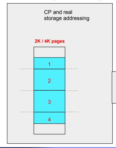
As the data addresses are in contiguous real storage, then one CCW data transfer command can be used for this I/O operation
