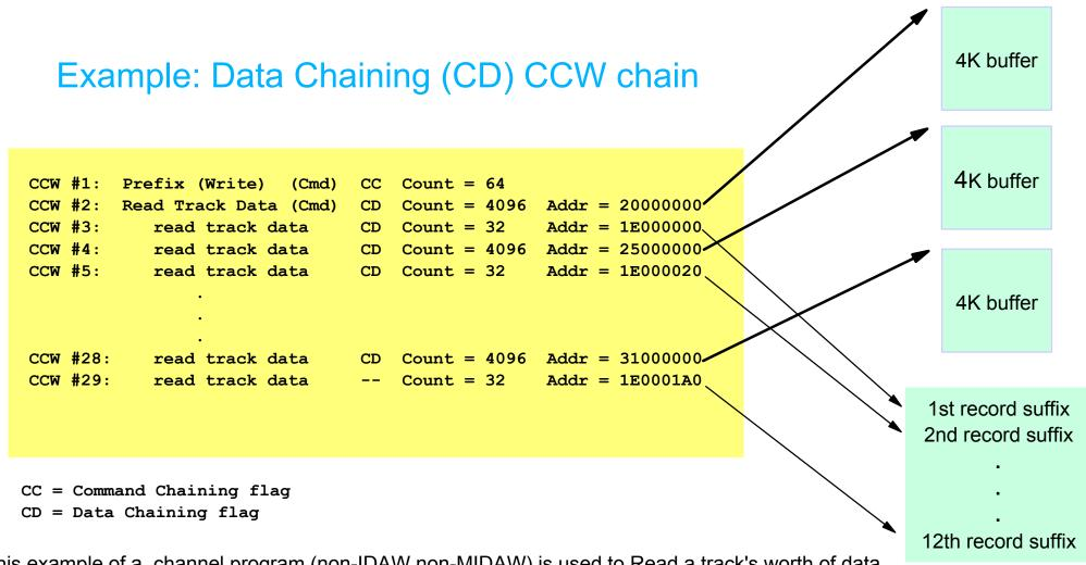
This example of a channel program (non-IDAW non-MIDAW) is used to Read a track's worth of data. Each record (software record) consists of 4K of data plus a 32 byte suffix.
