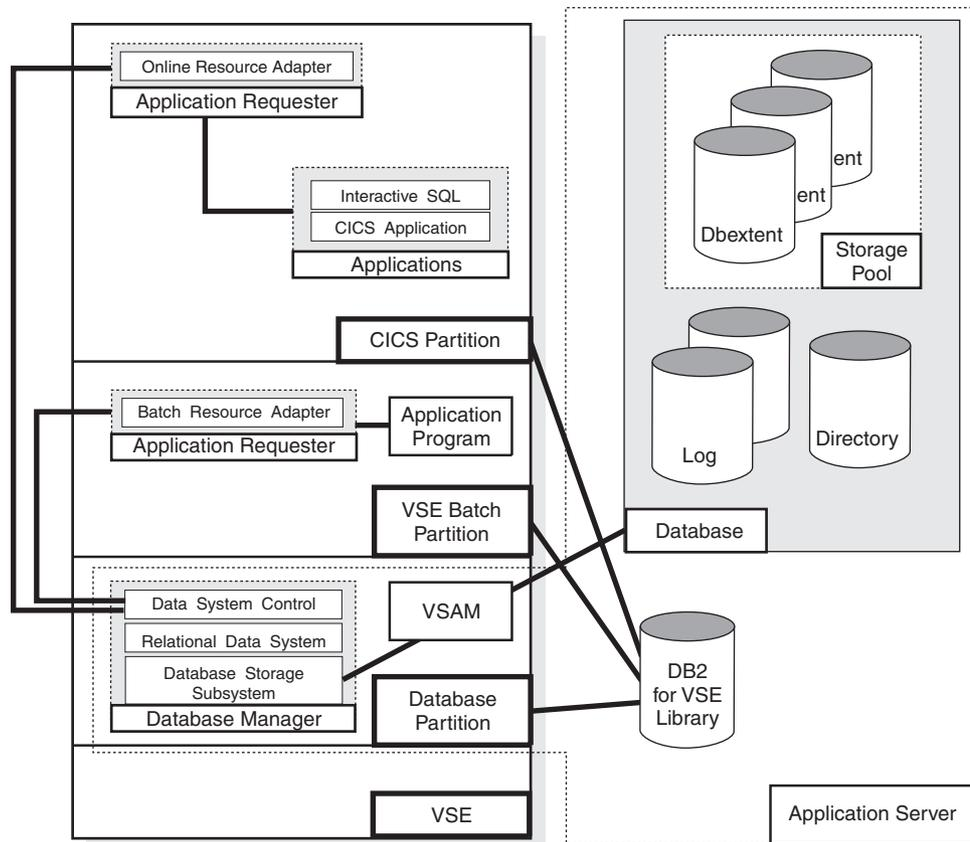
Figure 5. Basic Components of the RDBMS in VSE
