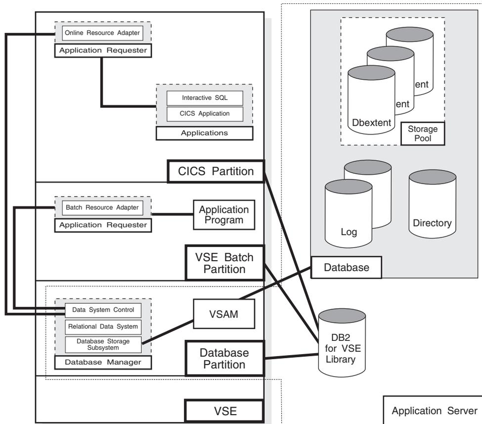
Figure 2. Basic Components of the RDBMS in VSE/ESA
