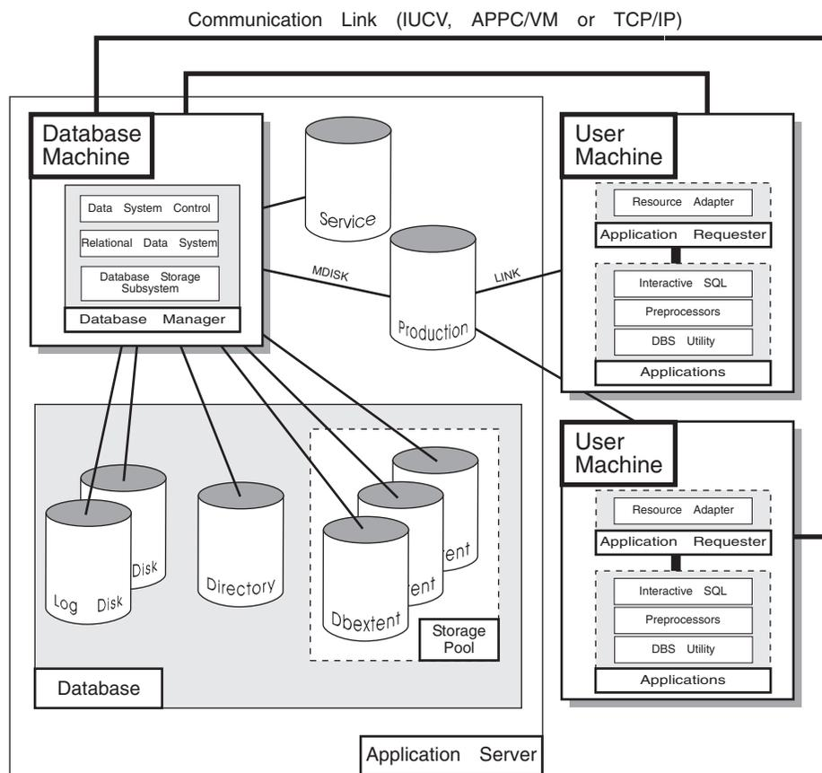
Figure 1. Basic Components of the RDBMS in VM/ESA
