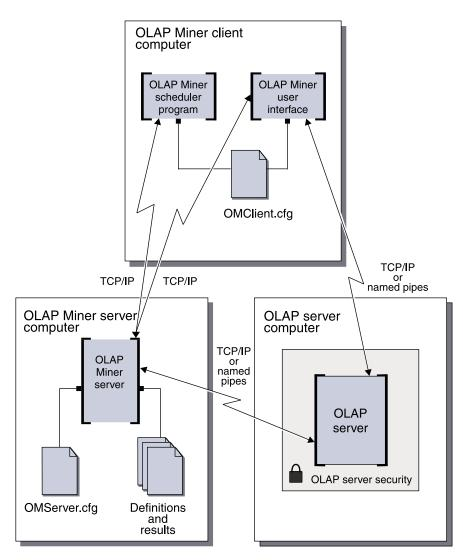
Figure 14. OLAP Miner system architecture
