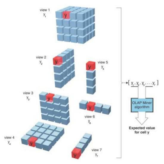
Figure 17. OLAP Miner computing the expected value for a single cell y
