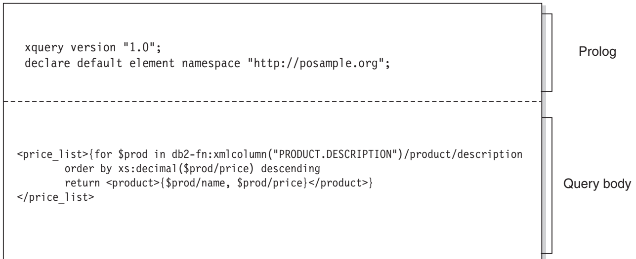
Figure 1. Structure of a typical query in XQuery
