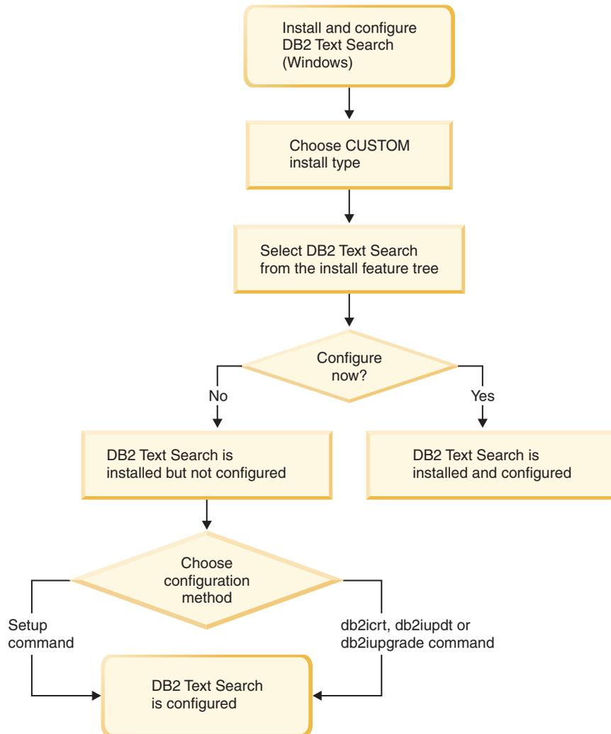
Figure 4. Installing and configuring on Windows platforms
