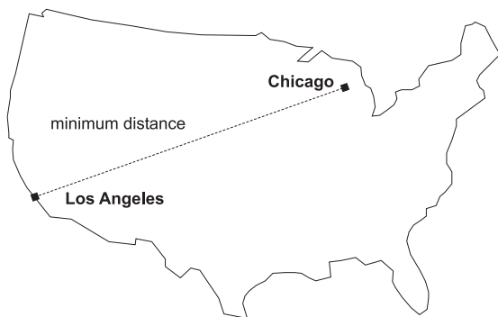
Figure 56. Minimum distance between two cities. ST_Distance can take the coordinates for the locations of Los Angeles and Chicago as input, and return a value denoting the minimum distance between these locations.
