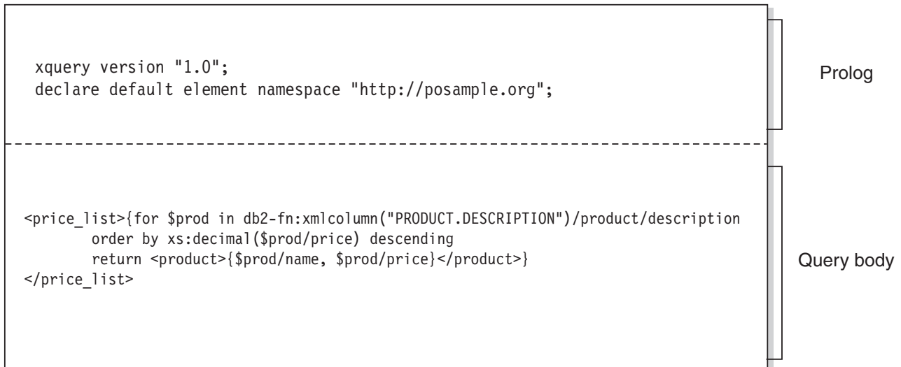
Figure 1. Structure of a typical query in XQuery
