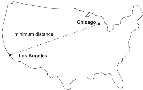
Figure 57. Minimum distance between two cities. ST_Distance can take the coordinates for the locations of Los Angeles and Chicago as input, and return a value denoting the minimum distance between these locations.
